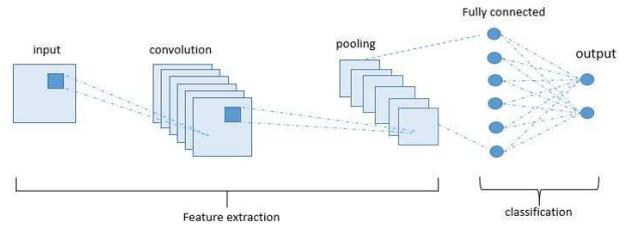
Fig. 3 The basic architecture of CNN algorithm.
