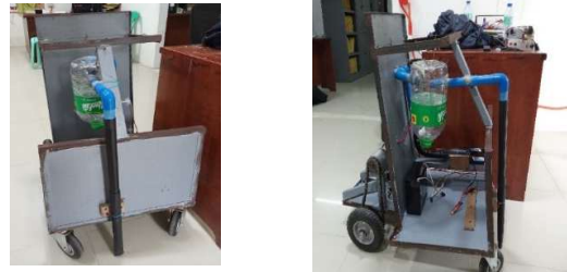
Fig. 11 Vacuum Suction and two-wheel drive feature of a Rice Grain Collecting Robot
