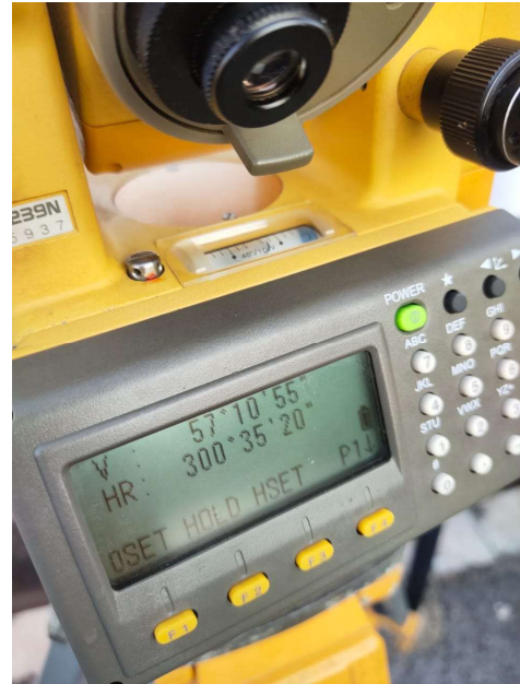
Fig. 2 Display and Key Panel of Total Station
