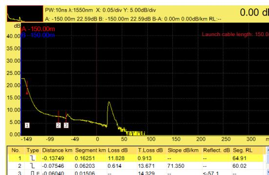
Figure 12. Testing OTDR using Adapter Barrel
