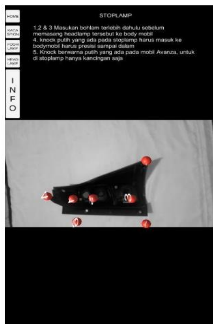
Figure 6. Stop Lamp AR Installation Tutorial
