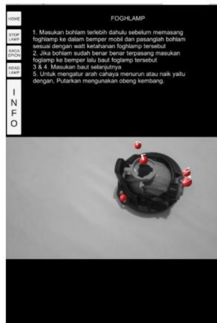
Figure 5. Fog Lamp AR Installation Tutorial
