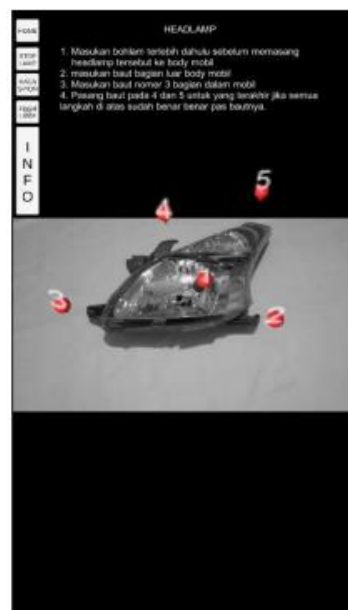
Figure 4. Headlamp AR Installation Tutorial
